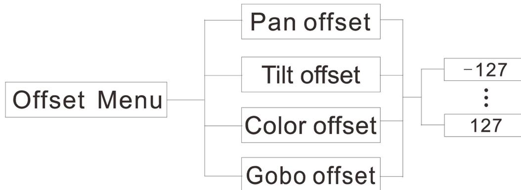
To enter the home position adjustment menu, press the ENTER button for at least 5 seconds. In this submenu you are able to adjust the original position of the pan position, tilt position, color wheel position, and gobo wheel position.
