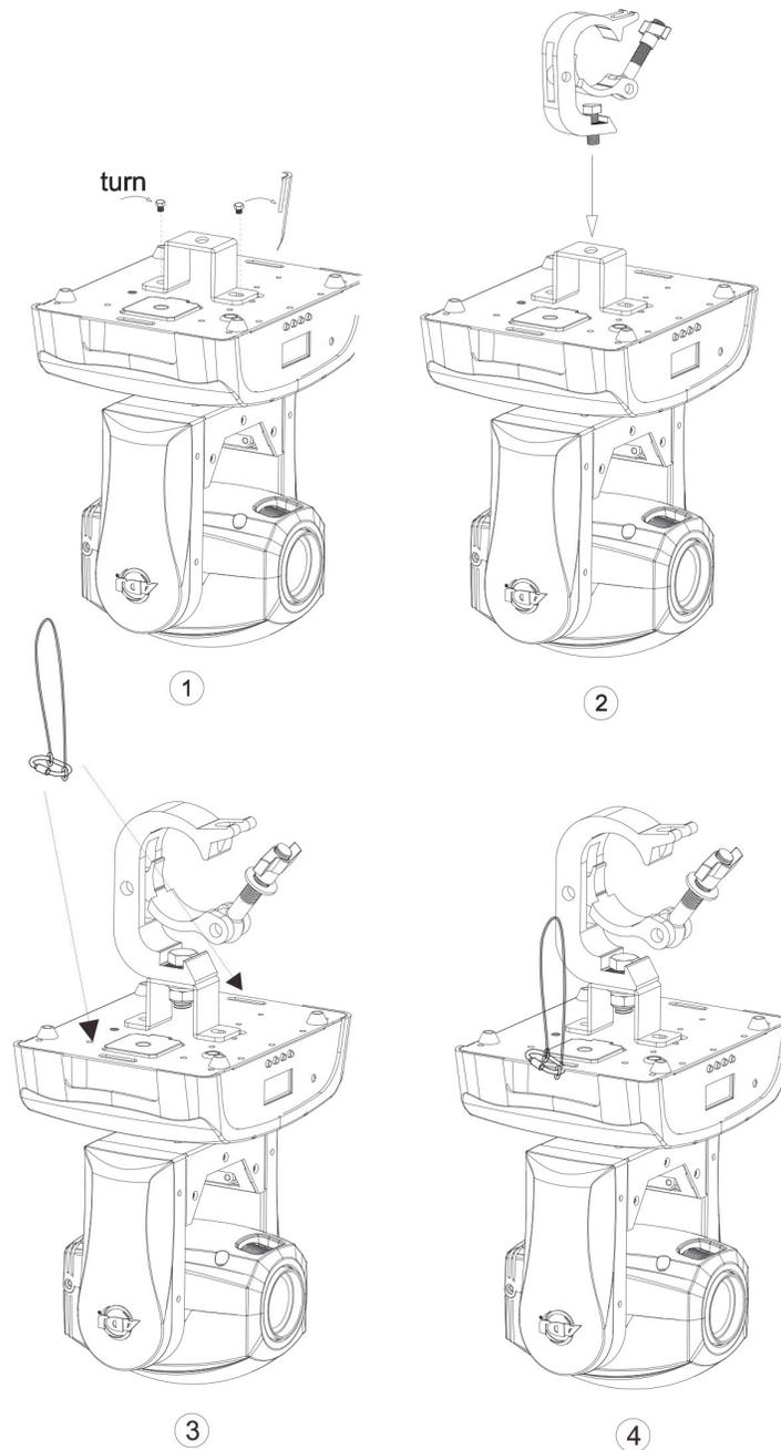
Screw one clamp via a M12 screw and nut to the included bracket. Attach the bracket using the included screws to the bottom of the Pocket Pro. Pull the safety-cable through the side holes located underneath the handles. Run the safety cable over the trussing system or a safe fixation spot. Insert the end in the carabine and tighten the safety screw.
