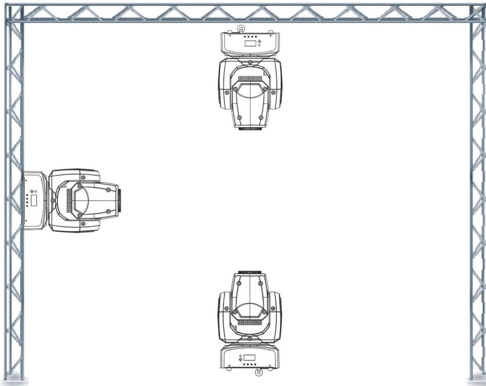
The Pocket Pro is fully operational in three different mounting positions, hanging upside-down from a ceiling, mounted sideways on trussing, or set on a flat level surface. Be sure this fixture is kept at least 0.5m away from any flammable materials (decoration etc.). Always use and install the supplied safety cable as a safety measure to prevent accidental damage and/or injury in the event the clamp fails (see next page).
